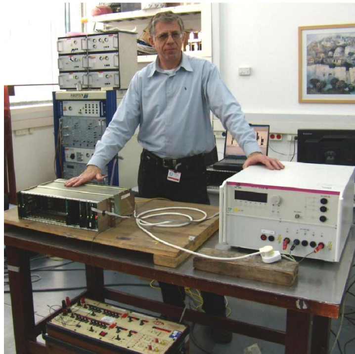
Fig. 16. The author in the process of testing the optical multiplexer (left) type FOCUS (Fiber Optic Communications for Utility Systems) for compliance with IEC standards for electromagnetic compatibility
